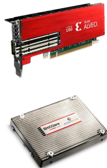
Figure 2: NoLoad enabled Xilinx Alveo U50 and Bittware 250-U2
